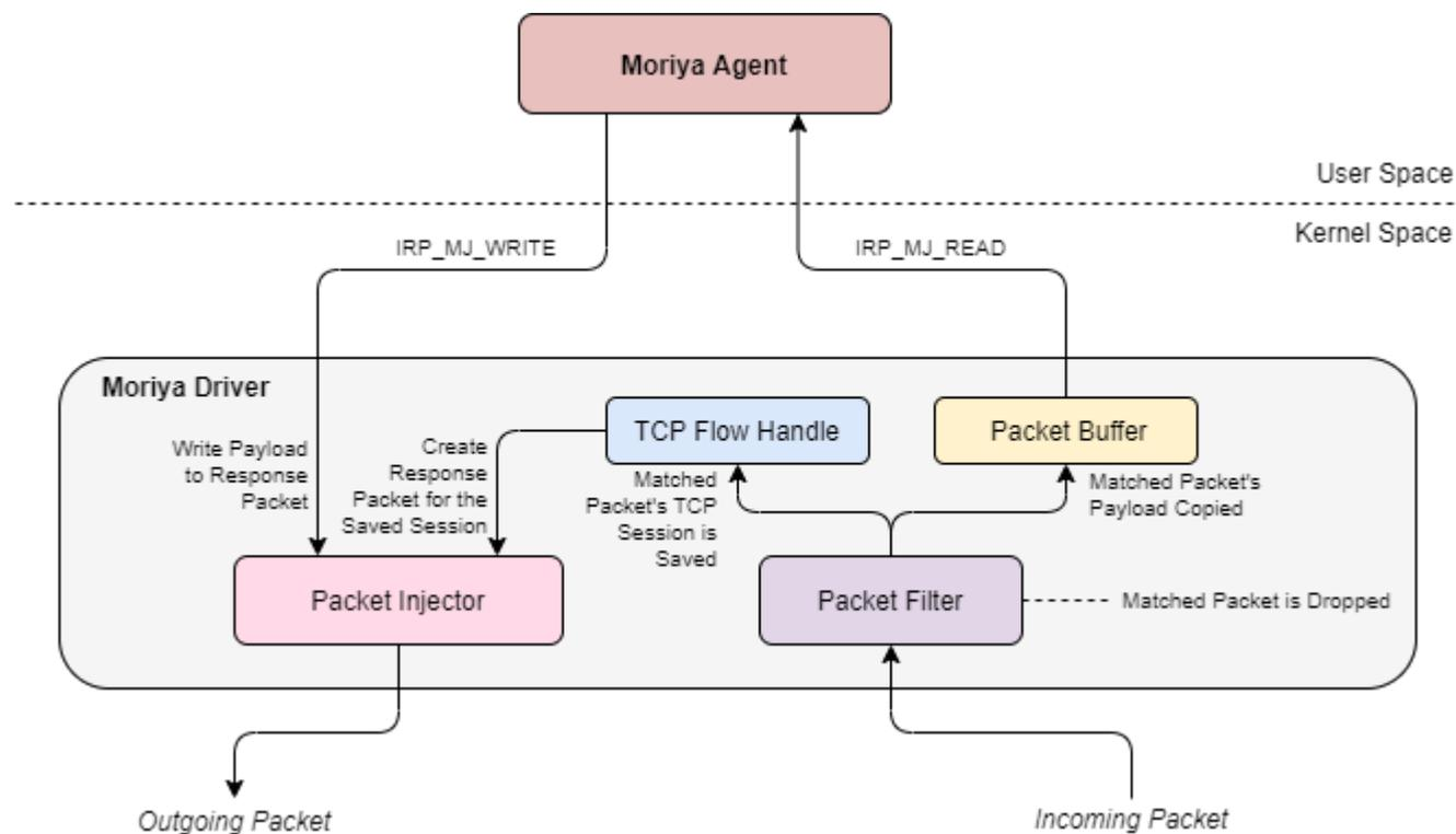
**Fig. 1. The architecture of the Moriya rootkit**
