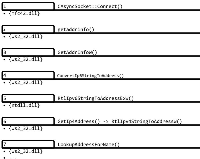
Figure 7: *CAsyncSocket::Connect()* API implementation sequence (Windows 7 ; 32-bit)
